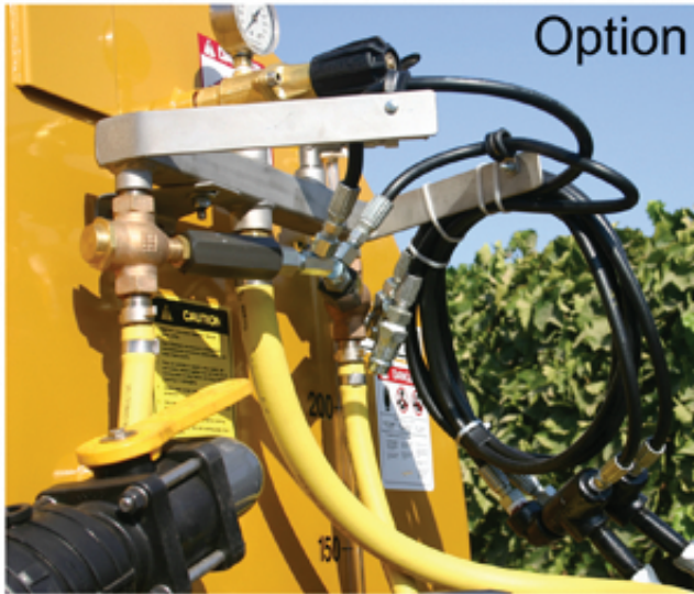
Dual Hydraulic Spray Valves
