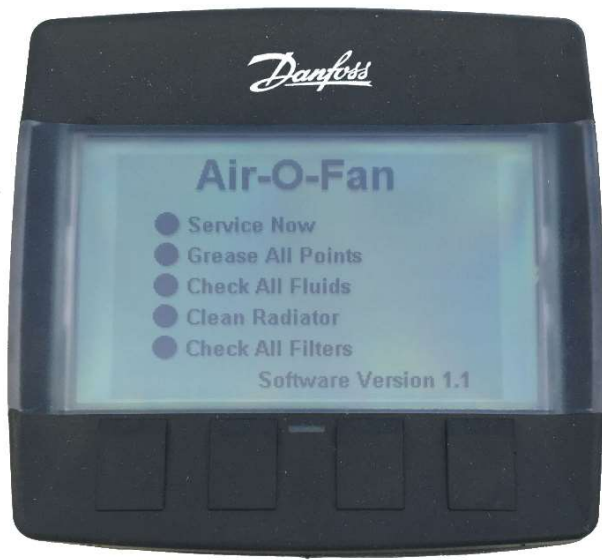
AIR-O-FAN Start Up Screen Display service maintenance and pre-start checks
