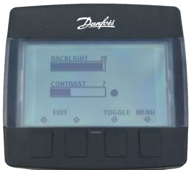
EDIT: Adjust Screen Values TOGGLE: Select Backlight or Contrast MENU: Return to Main Menu
